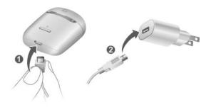
The internal battery starts charging. When hearing aids are inserted, they start charging as well. The charging status of the charger is shown permanently.
